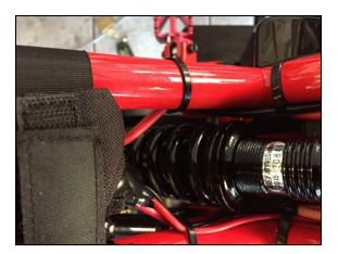
**Figure 2**. Solution of issue, all wiring securely cable tied to frame, well clear of rear shock unit.
