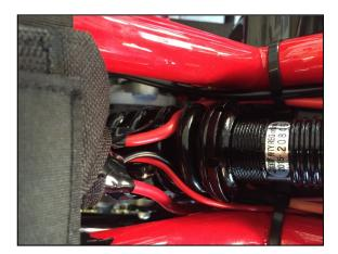
**Figure 1.** Potential issue of cable routing becoming caught in the coils of the rear shock spring.
